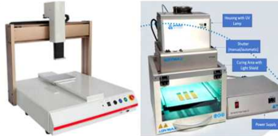
Fig 5 Glue Robot (Left), UV Equipment to Cure the Glue (Right)
