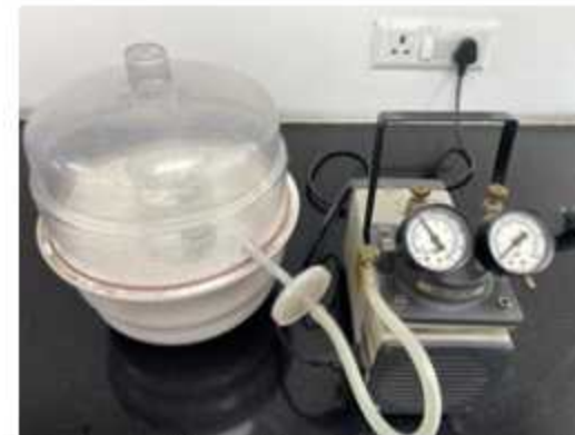
Fig 6 Vacuum Test (~500mmHg) on glued impellers.
