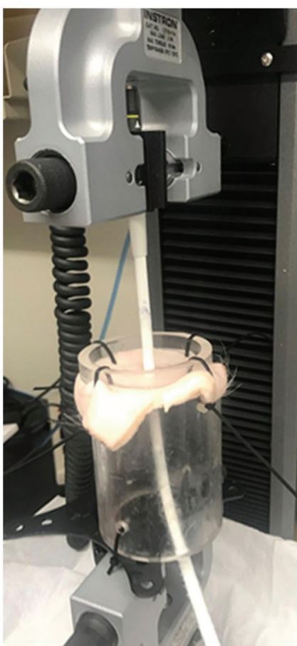
Figure 1. HeartMate driveline setup in fresh porcine abdominal tissue, connected to Instron tester. Angle from clear cylinder is derived from CT abdomen reconstructions of driveline tunneled tract length and angles.
