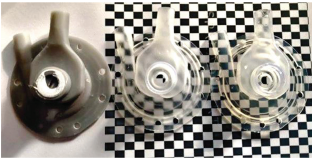
Figure 1.1. The translucent 3D printed part (left), transparent part prior to solvent polishing and final transparent part (right.)
